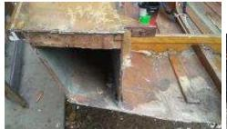
the new transom (including slot tabs to be on the safe side). A little tip when cutting ply, run masking tape along the pencil line so that when you cut with your jigsaw it does not splinter the wood. It works!
